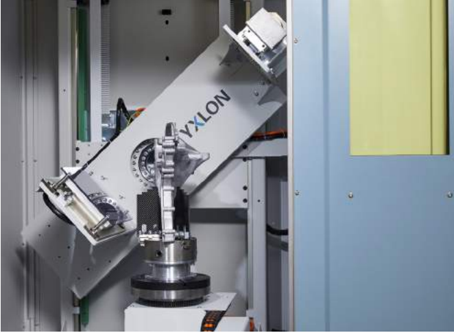
Large inspection envelope with multiple manipulation possibilities of part and x-ray components
