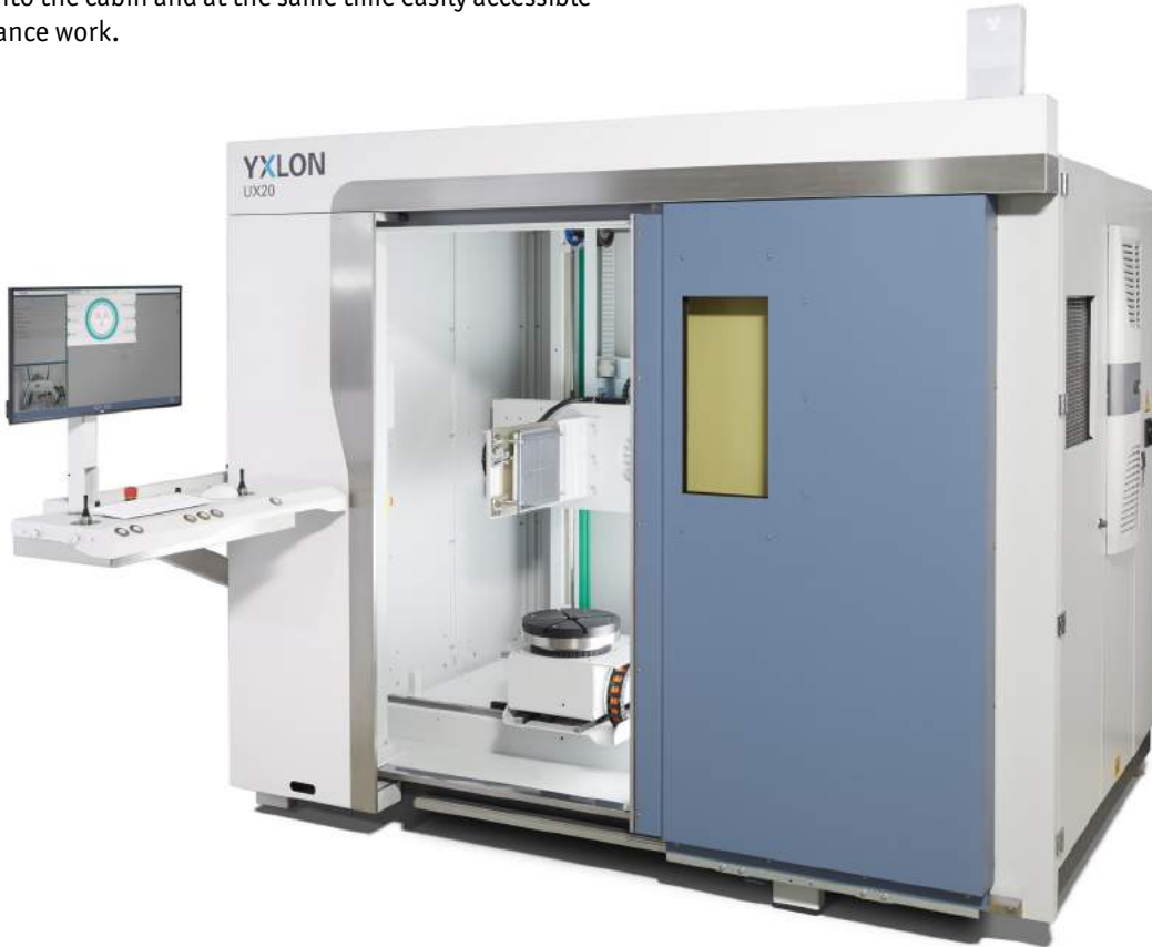
YXLON UX20 – compact radiography and CT system with clearly arranged and height-adjustable control desk
